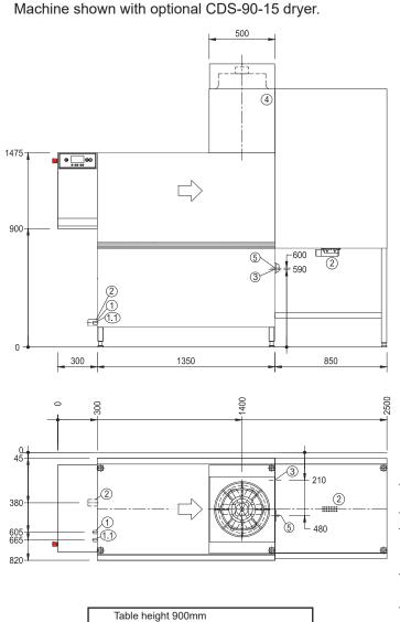
Machine height +/- 25mm feet adjustable
