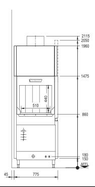
Warm water connection (filling) R 3/4" 0 - 3°d, (1,4mmol/l); 55-65 degrees Celcius 1.1 For machine operation Warm water connection for machine without heat recovery Cold water connection for machine with heat recovery R 3/4" 0 - 3°d, (1,4mmol/l); max. 260 l/h; demineralized water blended to have appr. 80 µs/cm Drain DN 50 415/50/3 N+E Power supply Without dryer - 28.7kW / With dryer (D90) - 32.3kW approx. 600m³/hr Exhaust Main switch Table height 900mm
