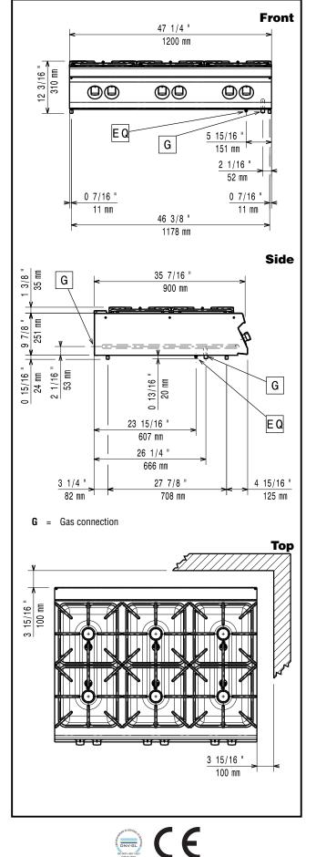
Modular Cooking Range Line EVO900 6-Burner Gas Boiling Top, 10 kW
