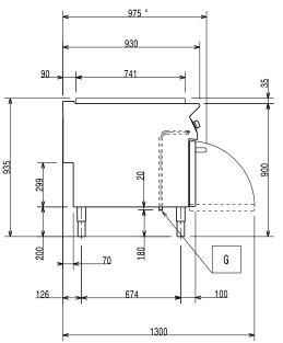
EQ = Equipotential screwG = Gas connection
