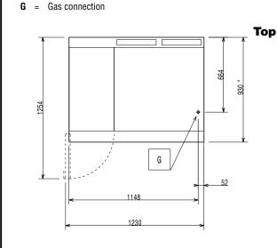
Modular Cooking Range Line EVO900 Gas Solid Top on Gas Oven with 2 Burners on cupboard
